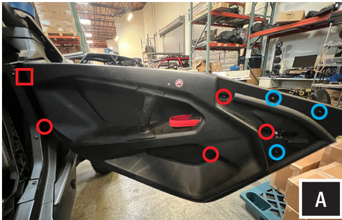
A. Remove the (3) T20 and (5) T30 Torx screws on the door panel. [A1] Note that the fifth T30 Torx screw is hidden behind the weather strip.
