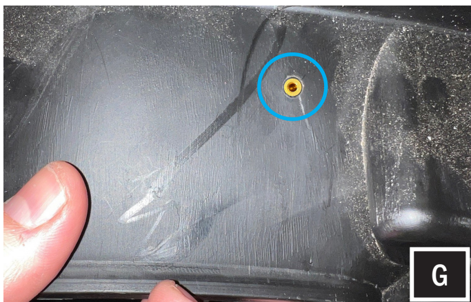
G. Line up the hole with the threaded insert on the speaker pod.
