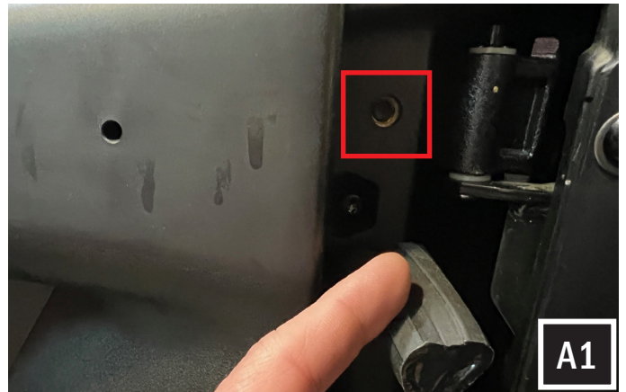
A. Remove the (3) T20 and (5) T30 Torx screws on the door panel. [A1] Note that the fifth T30 Torx screw is hidden behind the weather strip.
