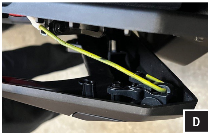
D. Unhook the door lock linkage rod to remove the trim.
