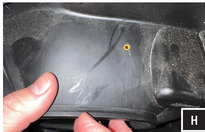
H. Use the provided screws and washers to secure the speaker pod. Do not fully tighten the screws yet.
