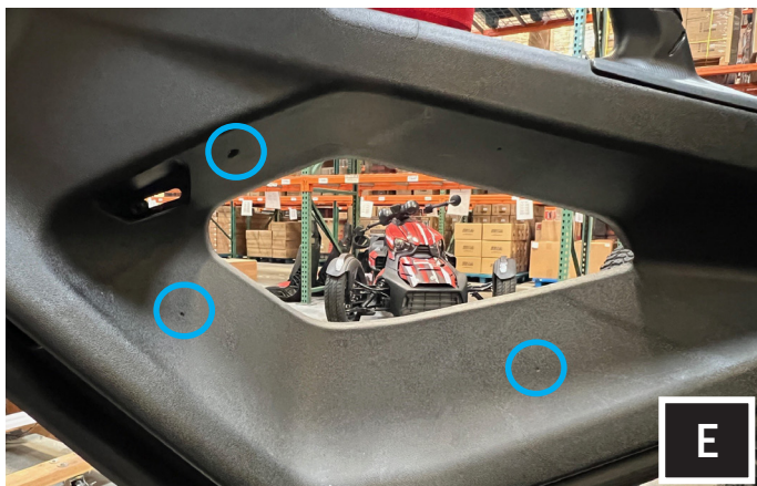
E. Drill out the (3) factory dimples using a 5/16" drill bit.
