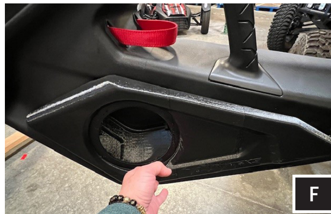
F. Hold the door pod while aligning the threaded inserts [G].
