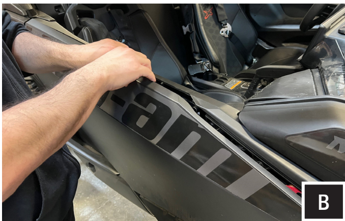
B. Carefully pop off the outer door skin starting from the top. [B1] Note that there are (2) clip fasteners on the top and (1) at the bottom.
