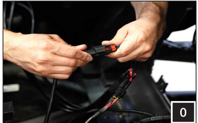
O. Plug in the B-H2936 (rear speaker harness) to the B-H1913 (4-pin audio extension harness, 8 ft.).
