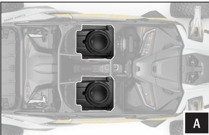
A. The MAVR-PHZ5VTD includes (2) subwoofer enclosures that are mounted under the driver and passenger seats.
