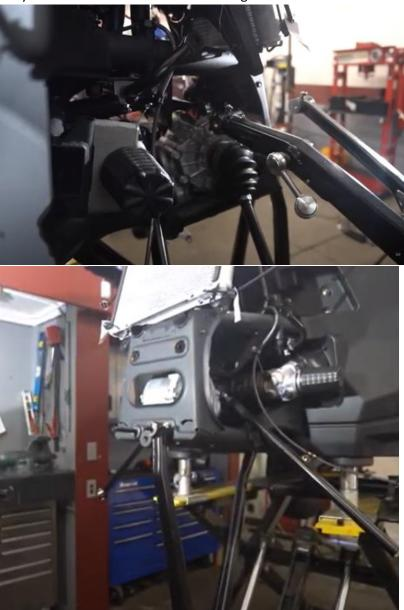
17. Remove 10mm bolts from between the lower control forward studs located on the front of the frame.
