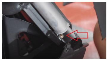
3. Once the vehicle is lifted using a jack, remove the 2 front shocks from the vehicle.
