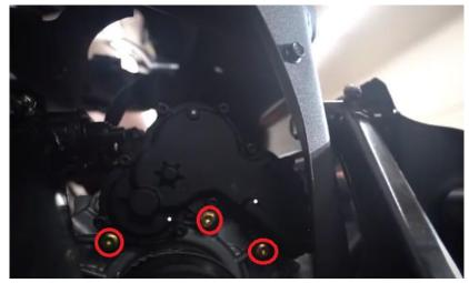
12. Drill out the 3/16" rivets on the lower A-arm holding the brake line. Sometimes are hammer and chisel are required to fully remove the rivets. Use special care not to damage brake lines or clips. Remove 10mm bolt at the bottom of the control arm to free the brake line.
