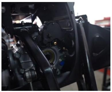
29. Reinstall axles to the vehicle and through the knuckle.
