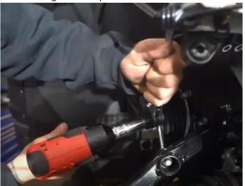
11. To gain access to upper control arm bolt, remove the smart -lok differential module by removing 3 torx T40 bolts. Once the bolts are removed, move the module up and out of the way. BE CAREFUL with module.
