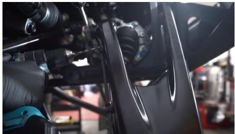
13. Remove upper and lower control arm front bolts.
