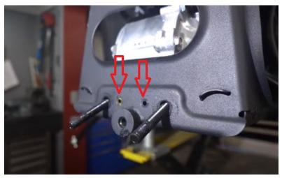
18. Begin by LOOSELY installing the upper control arm forward and rear plates. Each bracket is held in place with a provided nut, bolt, and a washer on each side.
