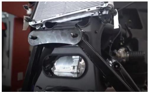
24. Replace bulk head and install nuts on forward upper and lower control arm bolts. Re torque to factory specifications.
