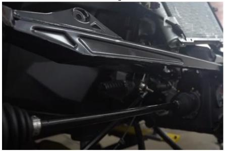
30. Reinstall lower A-arm to the knuckle using loc-tite.
