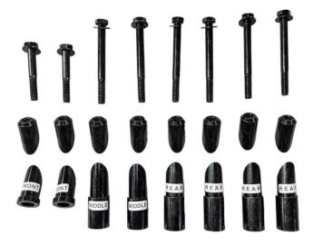
• Lay everything out on a clean scratch free surface and then divide up the hardware for each rocker guard so that each side has 2 rear standoffs and then the middle and the front get 1 standoff each, there are two shorter bolts included in the hardware bag and these go into the front mounting points only.
