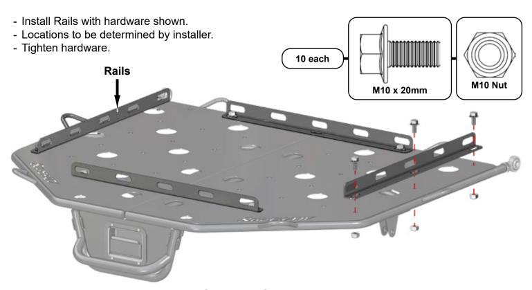
(use 3 sets of hardware for side Rails installation)
