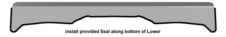
To ease installation, soak Seal in hot water before cutting or installing to increase flexibility.
