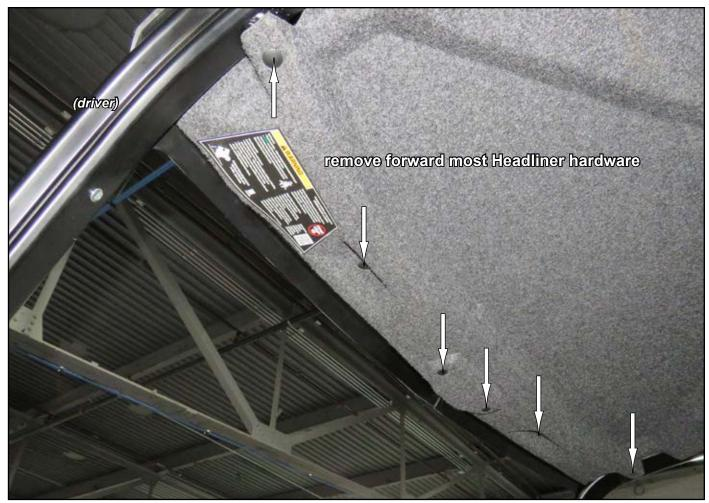
Resecure Headliner after Windshield installation has been completed.
