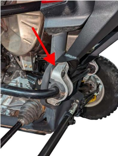
With the assistance of another person, hold the bumper up to the back of the vehicle and align the lower mounting points with the sway bar links mounting area and loosely mount the sway bar mount to the vehicle. The upper support rods will go to the underside of the bumper and secure with the supplied button head bolt, leave everything loose for now and the bumper can hang on it's own.
