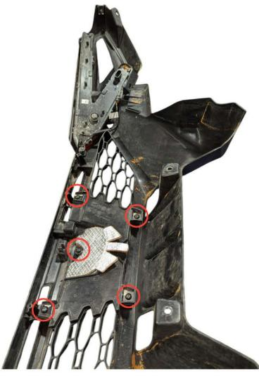
Lay the whole rear plastics assembly onto a soft surface face down, remove the camera connector end from the push mount it is attached to and discard of the push-in piece itself. While keeping the edge clip connected to the cameras harness, carefully pull upward on the clip and release it from the vehicle's plastic. Remove the 5 T20 torx bolts from the center of the plastic and lift away the camera and plastic panel as an assembly.
