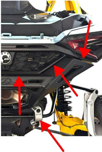
Once all the hardware is started shift the bumper as needed to get in lined up with the vehicles plastics and get the bumpers gaps between it and the vehicle nice and snug, from there tighten the upper support rods hardware at both ends first and then the lower mounts second.
