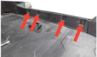
Remove the two lower T30 torx bolts located right above the exhaust exit followed by removing the 4 torx bolts located on the back edge of the cargo area on the vehicle. Support the rear section of plastic prior to removing the last couple torx bolts to prevent it from falling, carefully remove the plastic from the vehicle by pulling it toward the rear and away.
