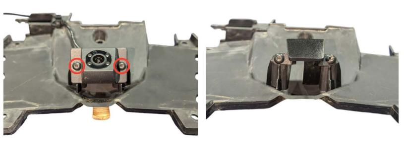
Remove the 2 torx bolts securing the camera to the plastic panel and remove the camera, with the supplied camera block off mount it to the panel as shown in the image above with the same hardware just removed.
