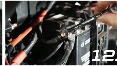
12. Locate the Dual 4AWG battery cable. Connect the black side of the Dual 4AWG ground wire to the ground on the OEM battery as shown
