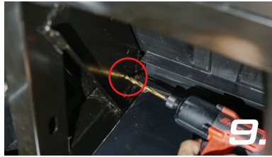
9. Drill back vertical hole to 1/2" for insert of nut and bolt
