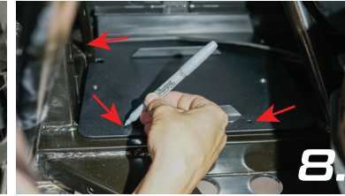
8. Insert battery mount in proper position inside driver's rear fender area. Mark 3 hole locations with a Sharpie
