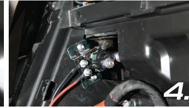
4. Attach ring terminal side of the Red/Black Trigger Harness to the battery isolator.
