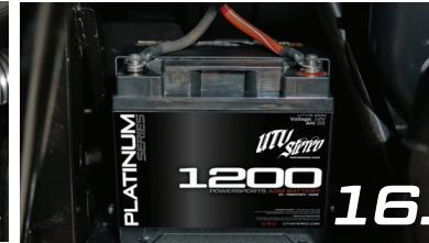
16. Connect 4AWG battery cable to UTVS1200 Battery
