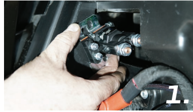
1. Hold UTVS Battery Isolator in place and make 2 marks with sharpie for mounting holes.
