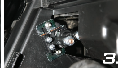
3. Use Supplied bolts to mount the isolator to the plastic, with installed Clip-On Barrel Nuts.
