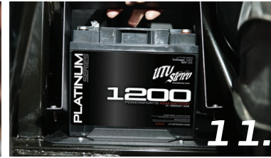
11. Install UTVS Battery and fasten with battery strap. Attach strap to the mount with supplied bolts. Screw bolts into the mount through pre-installed nuts
