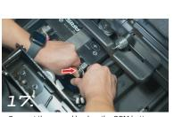
Connect the ground lead on the OEM battery
