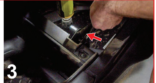
3 REMOVE BOLTS FROM SEAT MOUNT ON BOTH SIDES
