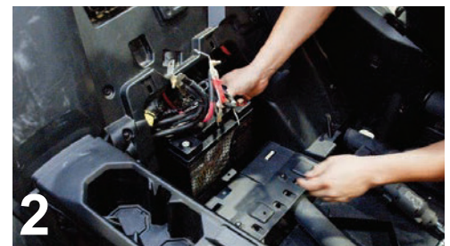
2 PLACE THE BATTERY IN THE VEHICLE
