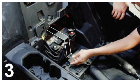
3 PLACE THE TOP BRACKET OVER THE BATTERY AND MAKE SURE THE HOLE ALIGNS WITH BOTTOM BRACKET
