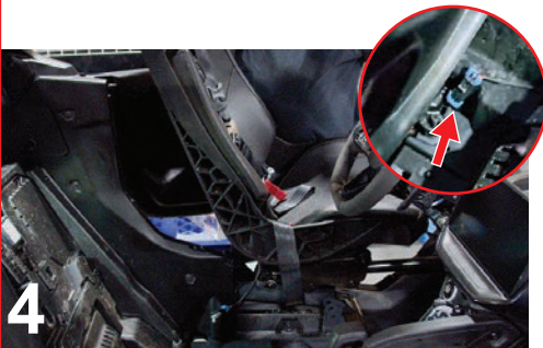
4 LIFT SEAT UP TO GET TO THE BLACK SEAT BELT PLUG AND UNPLUG IT
