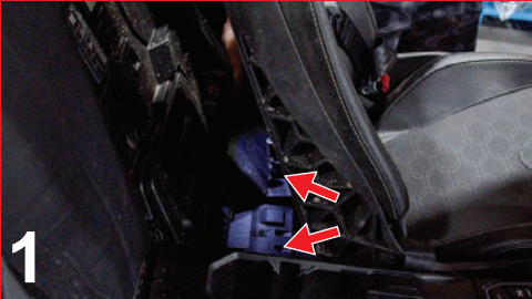
1 SLIDE SEAT FORWARD AND REMOVE BOTH BOLTS FROM FLOOR
