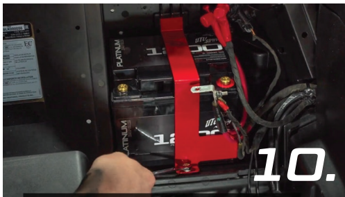
Place the top bracket onto the battery and connect the brackets using the included bolt
