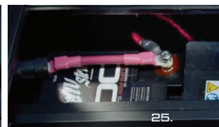
25. Connect SHORT red lead and any aftermarket accessories to positive terminal on 2nd battery
