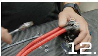
12. Place the LONG red wire on the other side and tighten securely
