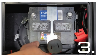
3. Remove the battery strap and pull the OEM battery out of vehicle
