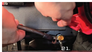
21. Loosen chassis ground bolt and attach 2nd battery ground wire Tighten securely
