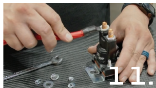
11. Place the SHORT red wire on the side shown here and tighten securely
