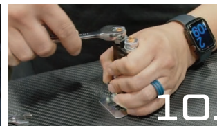
10. Remove ALL the nuts on the isolator
