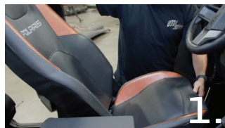
1. Remove the 2 bolts from under the driver's Seat. Remove seat from vehicle
