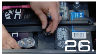
26. Take chassis ground wire and secure to negative terminal on 2nd battery
