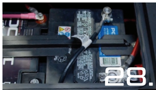
28. Replace positive lead on the OEM battery and secure LONG red lead to the OEM battery
